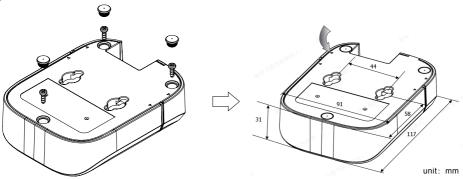
a. remove rubber plug and screws.
