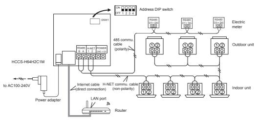
**H-NET communication cable** connects to H-NET terminal 1 and 2 of indoor unit and outdoor unit . **485 communication cable** connects to the RS485 end of electric meter. A connects to D1+, and B connects to D0-. **Internet cable** connects to LAN port of router (when adopted wired connection). **Power adapter** connects to the plug of AC100-240V. Select a proper AC plug according to actual onsite conditions.
